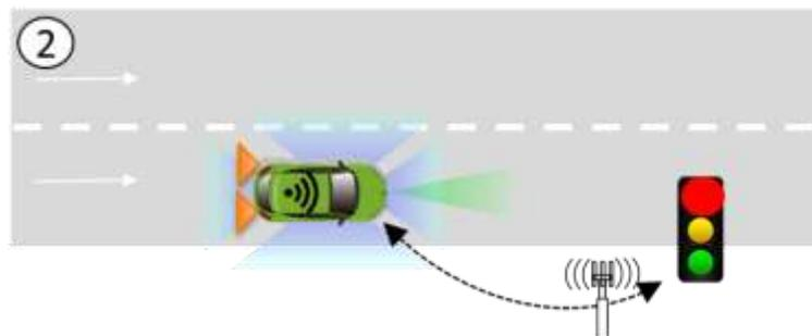
Figure 77: Automatic braking based on time to red information from traffic light
