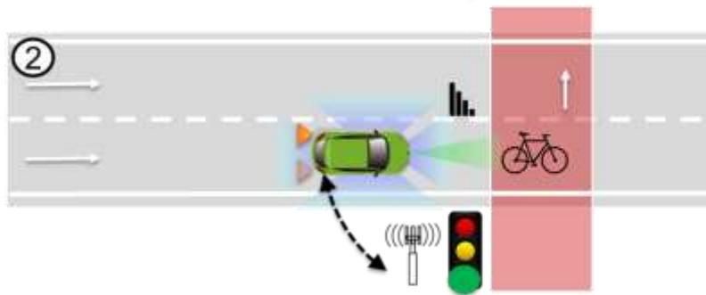
Figure 82: Braking in case of VRU traffic light violation
