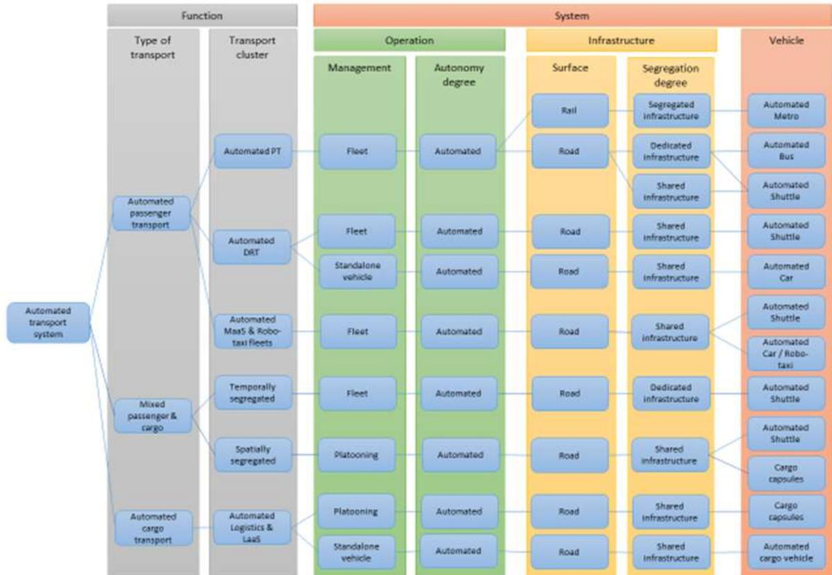
Figure 17: Automated transport systems classification modified from CityMobil2 project.
