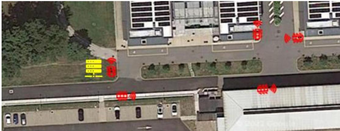
**Figure 3: Layout of the cooperative traffic lights and the road side unit installed at JRC Ispra by Swarco Mizar.**
