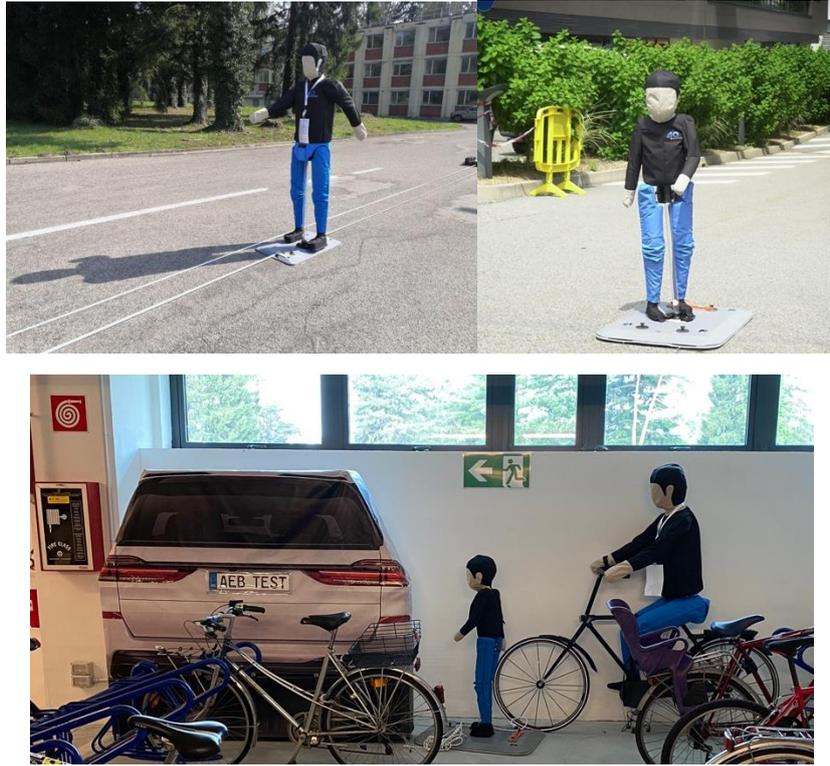
**Figure 4: Example of targets used for vehicle safety testing.**
