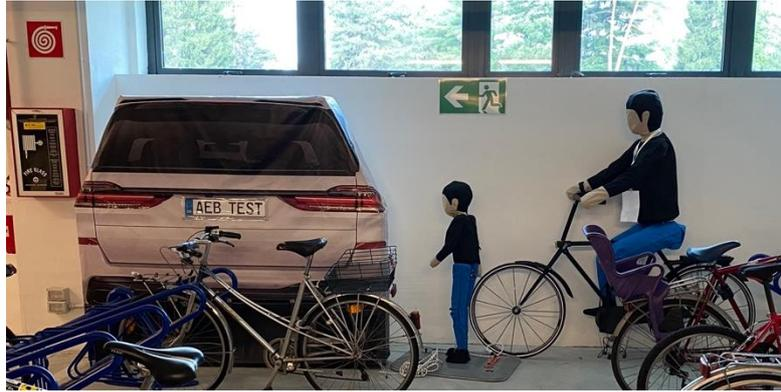
**Figure 4: Example of targets used for vehicle safety testing.**
