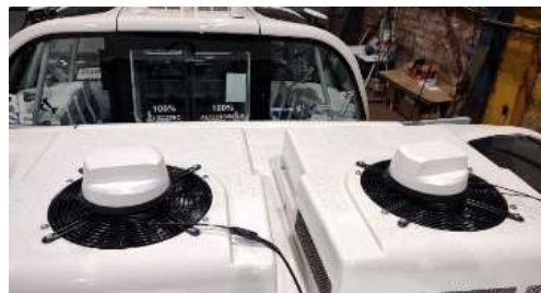
Figure 54: 5G vehicle antennas on the roof of the Navya shuttles
