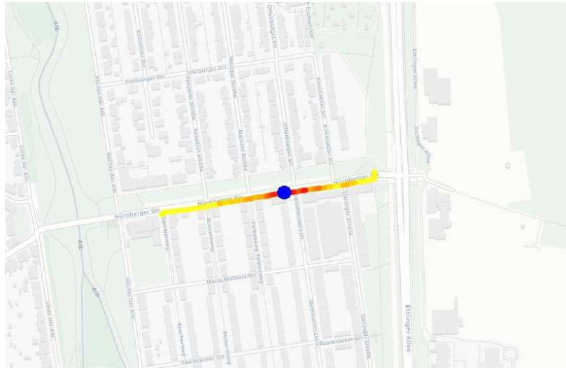
Figure 95: The RSSI of ITS-G5 based communication. Low signal strength is depicted in yellow, high signal strength is depicted in red, the position of the RSU is marked in blue (Lambing, et al., 2021).
