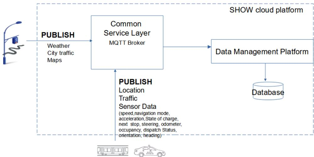
**Figure 23: MQTT APIs for ETA service**
