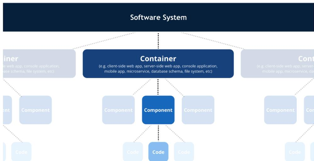
**Figure 32: C4 model main blocks' hierarchy (source: <https://c4model.com/>)**
