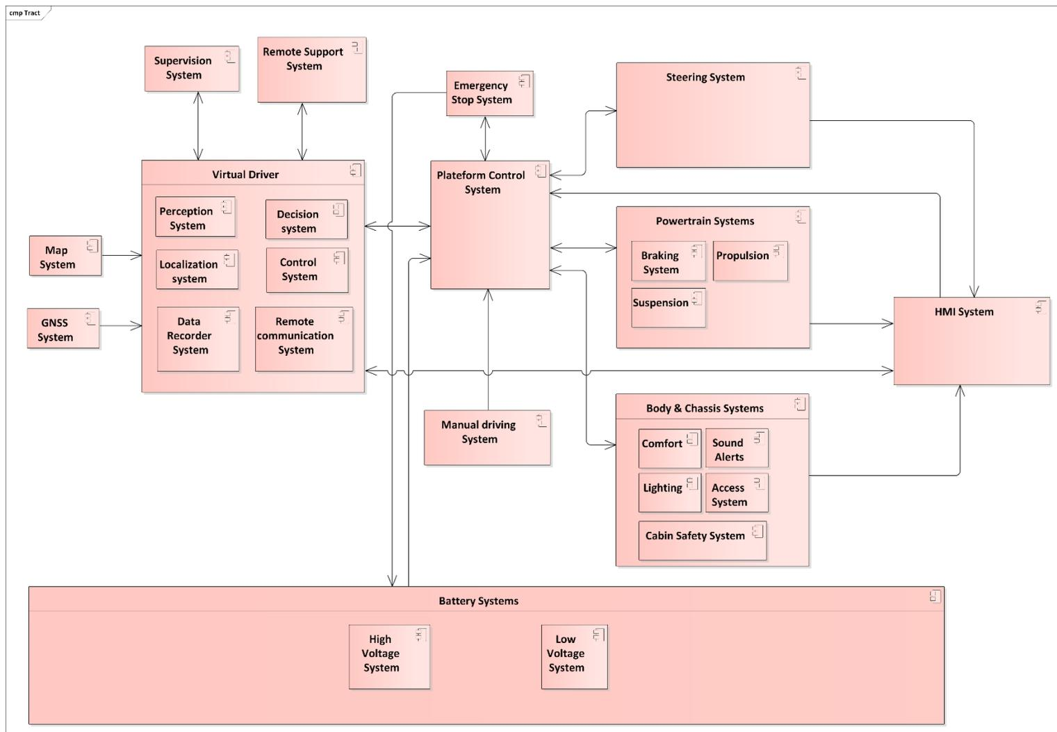
Figure 18: SHOW CAV generic functional on-board architecture.
