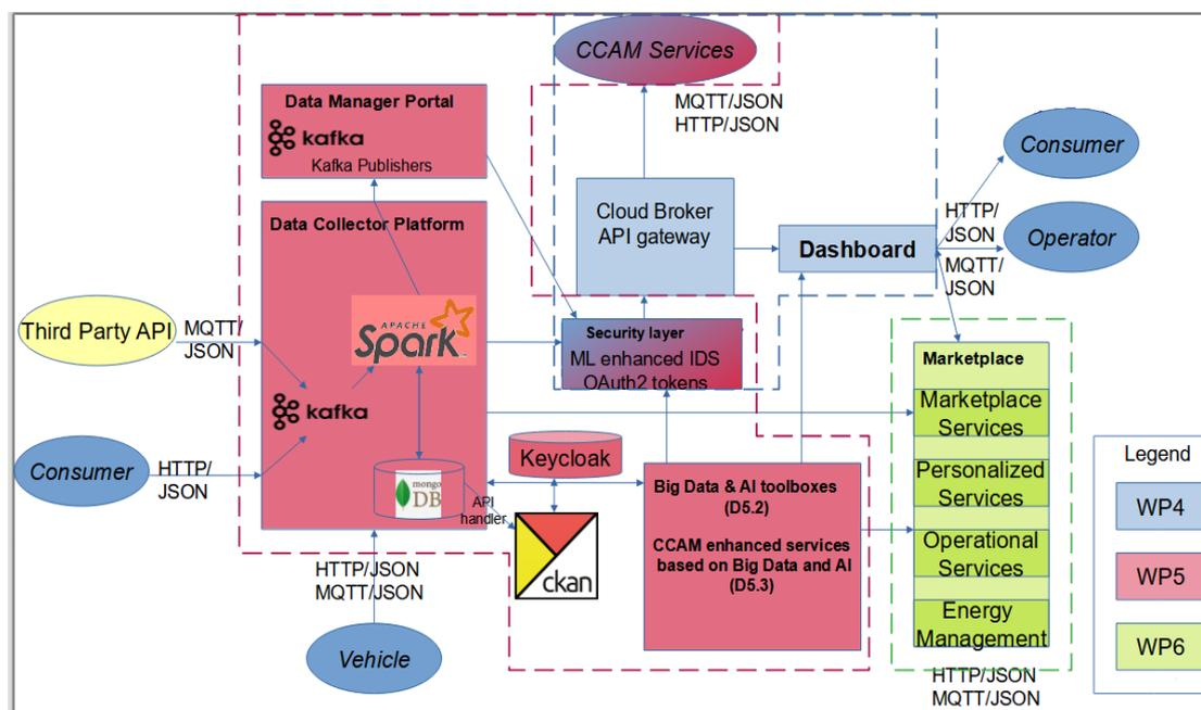
**Figure 19:** Inter-component relations of Data Portal and Big Data collection platform and their connection to SHOW web-services (source D5.1 [14]).
