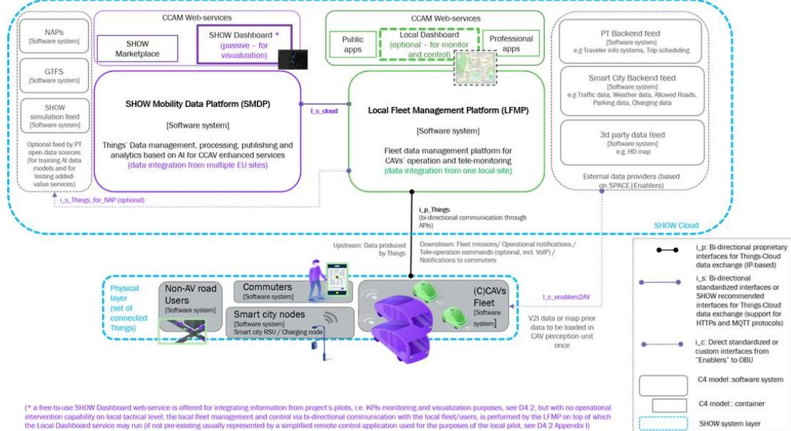
Figure 14: SHOW reference dashboard service and LFMP (demo site) dashboard service roles in the SHOW reference architecture (better viewed in zoom-in mode).
