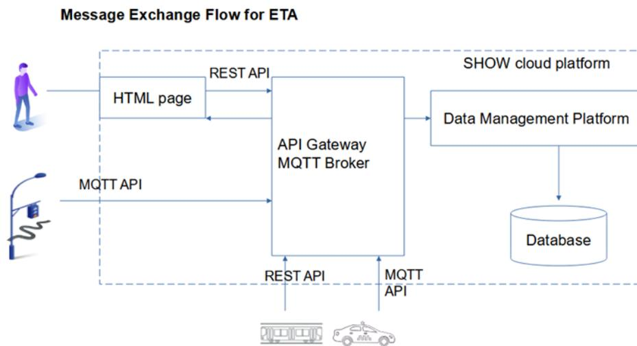
**Figure 22: Overall message exchange for ETA service**
