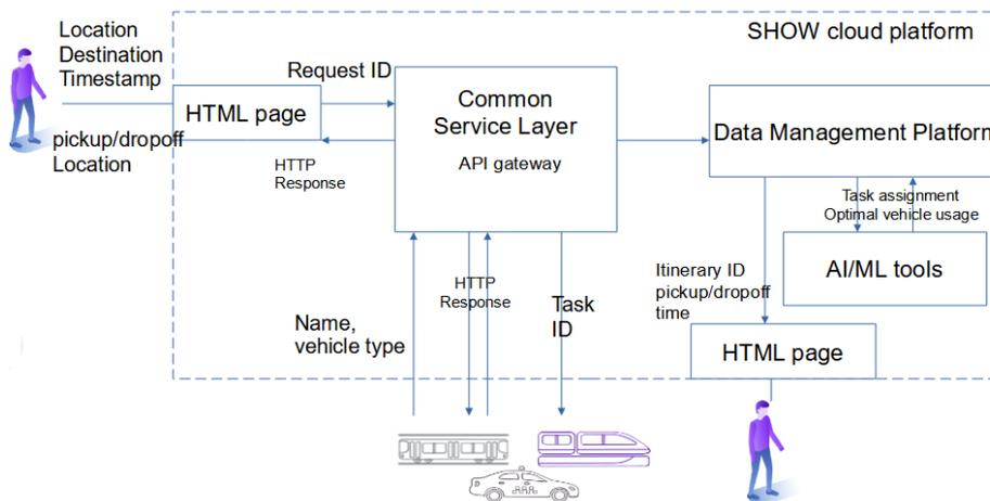
Figure 26: Message exchange for Multimodal Planner service via REST APIs and MQTT
