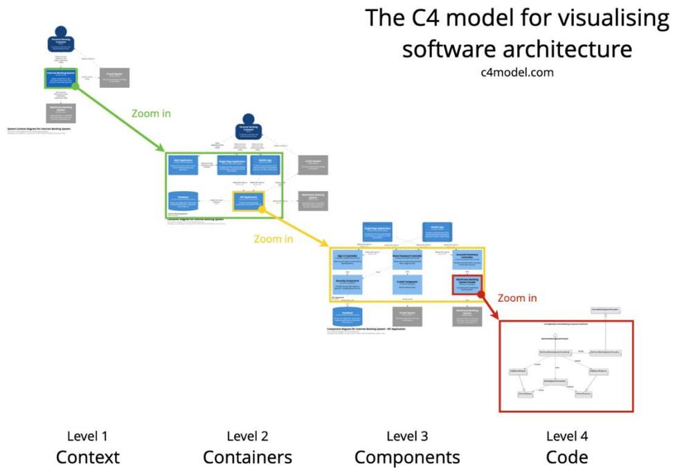
**Figure 31: C4 model levels of SW representation (source: <https://c4model.com/>)**
