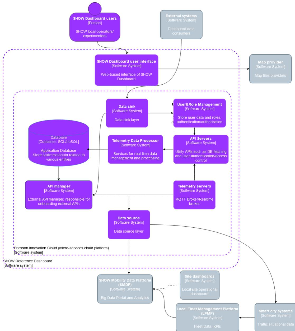
**Figure 21: SHOW Dashboard architecture diagram (Component level)**
