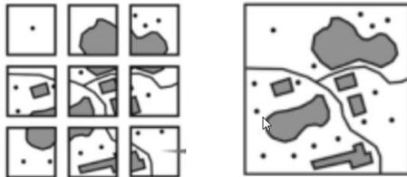
**Figure 4: Map constructed by a set of static images generated by a tile-server.**
