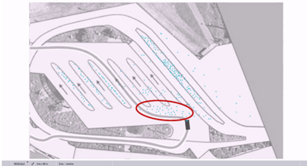
Figure 21: Screenshot of a simulation run showing the area (marked with a red ellipse) where the most conflicts between pedestrians and the AV occur.
