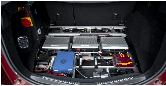
Figure 3: Retrofitted components in the TNO Carlabs trunk.
