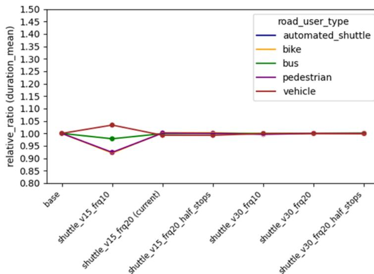
**Figure 23: Comparison of the relative ratios of the travel times between the scenarios at the Linköping site**
