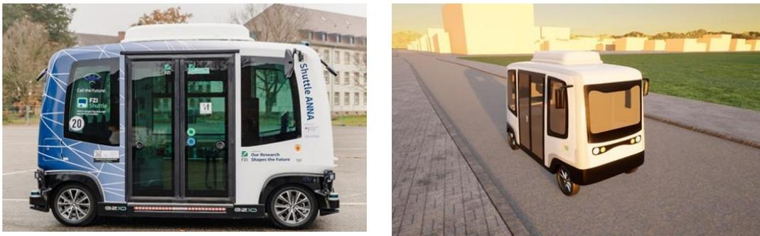
**Figure 14: Physical shuttle and blender model of the EasyMile EZGen2 shuttle**
