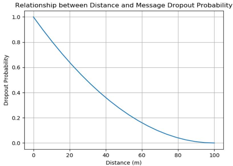
**Figure 17: Probabilistic dropout of messages**
