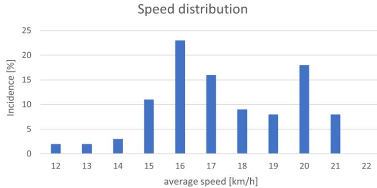
**Figure 8: Distribution of average speed over 100 simulation runs using SUMO**
