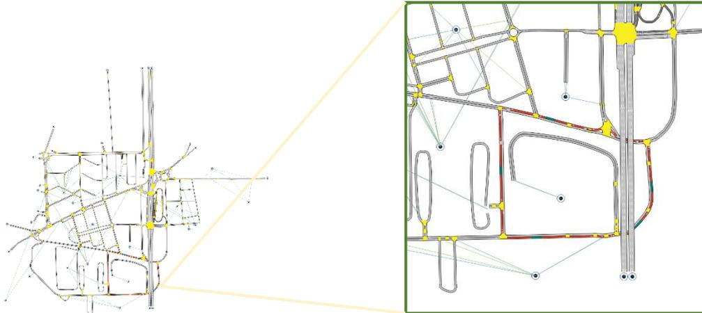
**Figure 25: Villaverde network in Aimsun Software with OD centroids (left) and circular route of SHOW automated shuttles, highlighted in red (right).**
