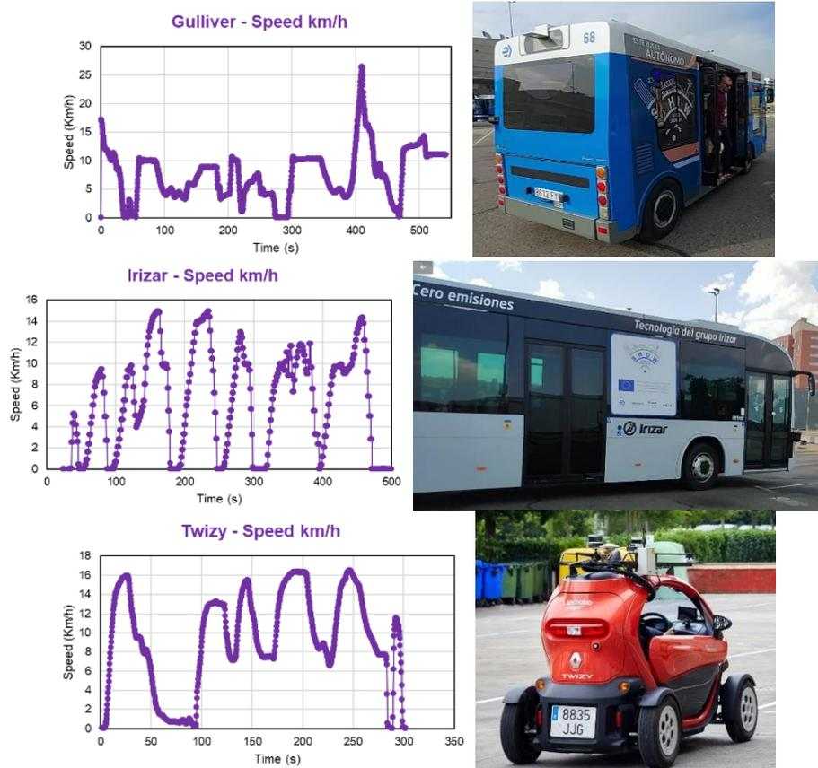
**Figure 31: Example of realistic speed profile from Gulliver, Irizar and Twizy operations.**
