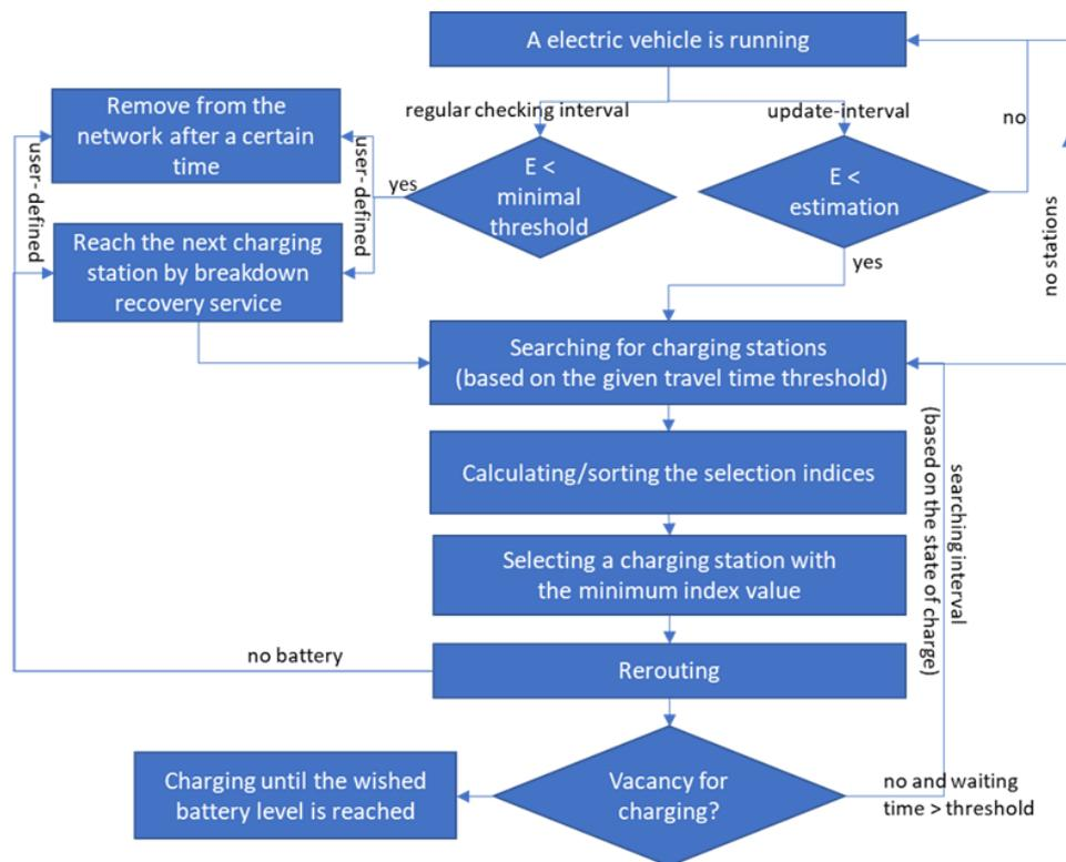
**Figure 20: The sketch of the proposed concept to model charging activities on the way**
