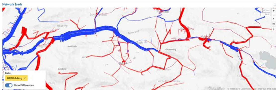
**Figure 47: Changes in network loads (number of daily vehicles traveling a long a link) from the base scenario to scenario G: The red lines mark increases in network load (due to DRT on minor roads) and blue marks decreases in network load (e.g., on the main road from the study area to Salzburg)**
