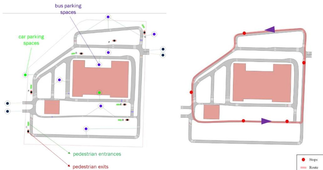
**Figure 29: Carabanchel network in Aimsun Software (left) and circular route with bus stops (right).**
