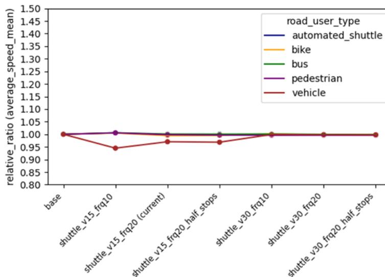
**Figure 22: Comparison of the relative ratios of the average speeds between the scenarios at the Linköping site**
