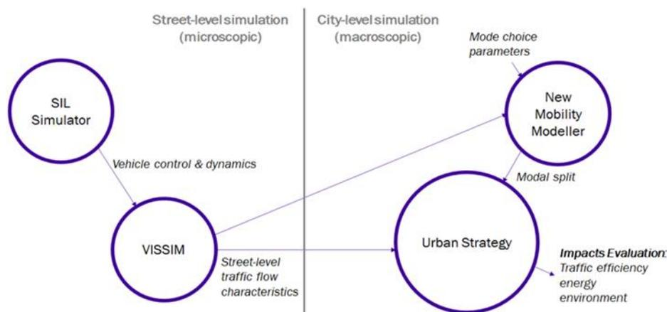
Figure 1: Overview of Brainport simulation architecture
