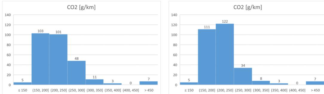
**Figure 11: Distribution of CO2 emission per vehicle without AV and with AV**
