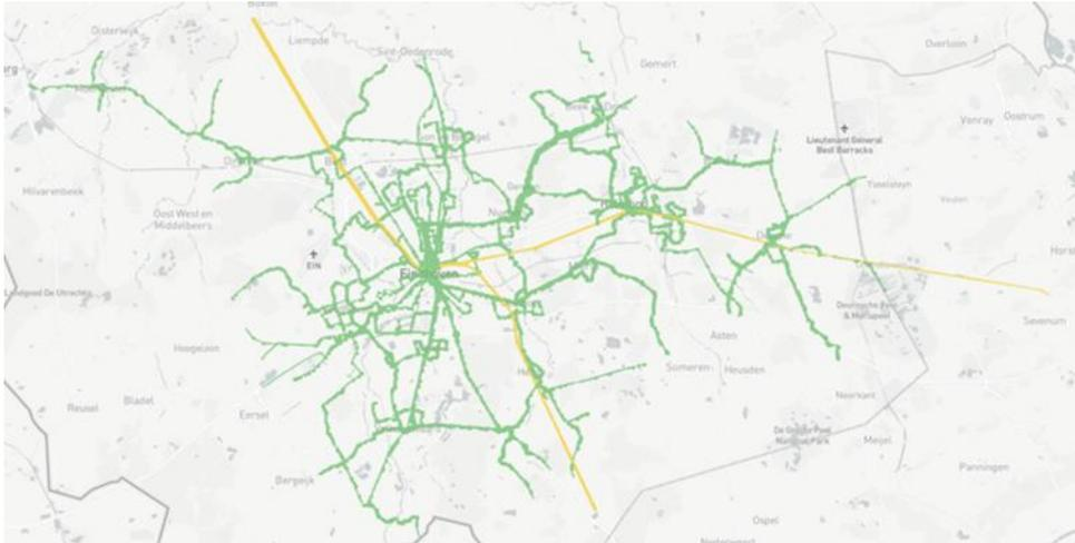
**Figure 2: Overview of transit lines (green: bus, yellow: train) in the simulation environment**
