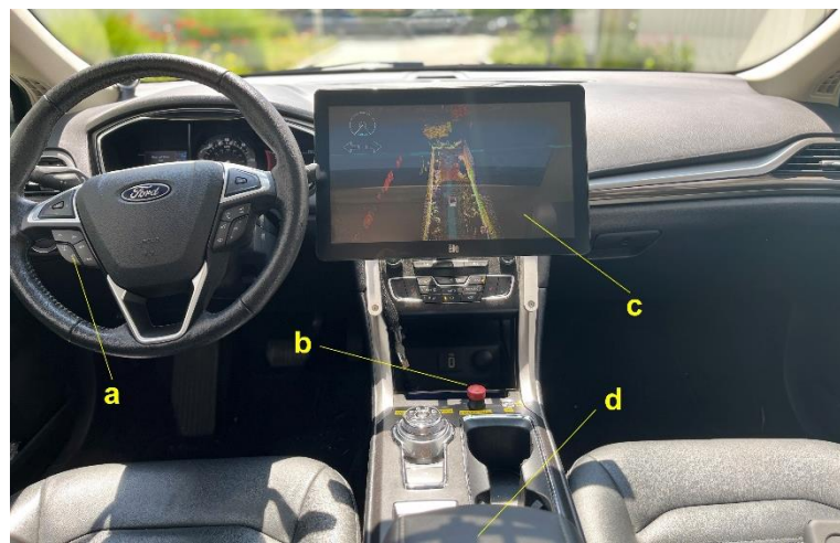
Figure 22: Buttons for activation of automated driving, (b) emergency stop button, (c) screen for test driver and (d) tablet for passenger (Source: Virtual Vehicle)
