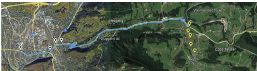
Figure 32: Road site units on the pilot track for automated vehicles in Koppl (yellow) and on the C-ITS enabled bus corridor (blue line) into the city of Salzburg (Source: Kapsch TrafficCom; adapted by Salzburg Research)
