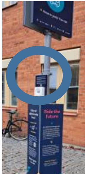
**Figure 5: Simple stop buttons placed at each bus signed bus stop, showing the shuttle operator if passengers are waiting at a specific stop** (source: My Weidel/VTI)
