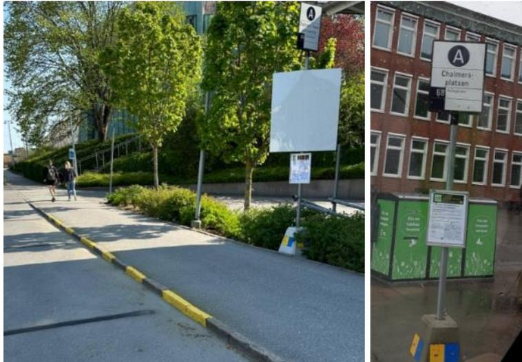
**Figure 33: Shuttle stop at Chalmers transport south with a LiDAR marker (white rectangle) and at Chalmersplatsen without LiDAR marker (source: Keolis)**
