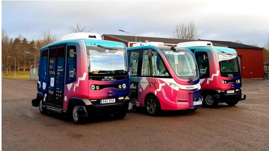
**Figure 7: The three AV shuttles in Linköping. The middle shuttle is a Navya DL4 Arma, the two on the sides are EasyMile EZ10 Gen2 (source: My Weidel/VTI)**
