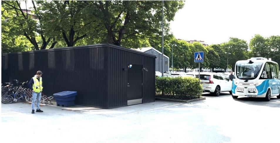
**Figure 43: VRU testing. Lights on vest informing and drawing attention to that the automated shuttle is approaching.**
