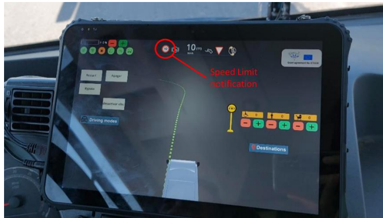
Figure 3: Madrid Mega site: AV HMI used and speed limit notification visualization.
