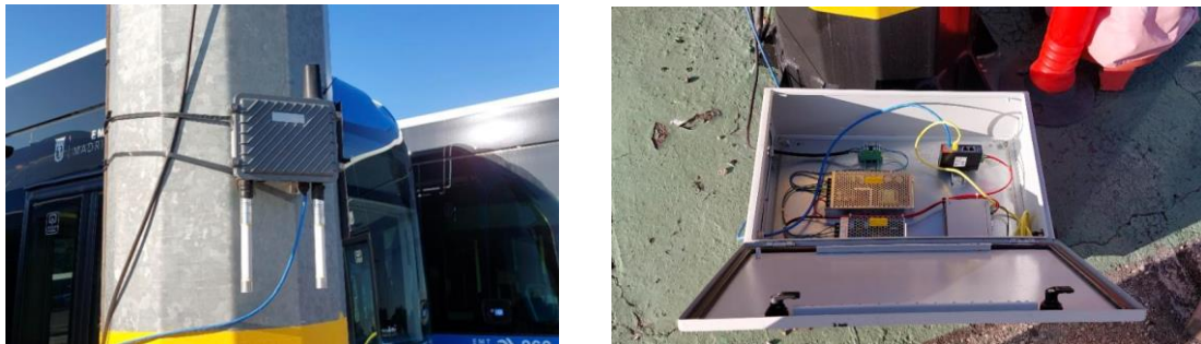
Figure 2: Madrid Mega site: Speed limit C-ITS service RSU equipment deployed
