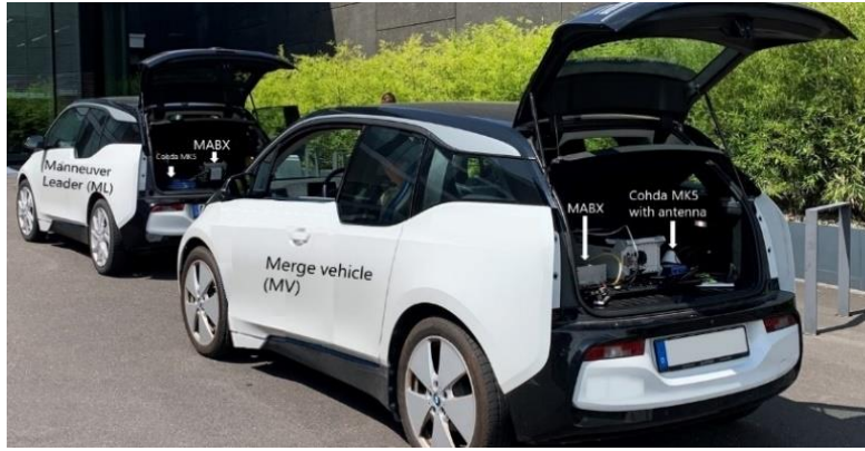
Figure 14: Two automated vehicles equipped with Micro Autobox and Cohda MK5 communication units (source: FEV)
